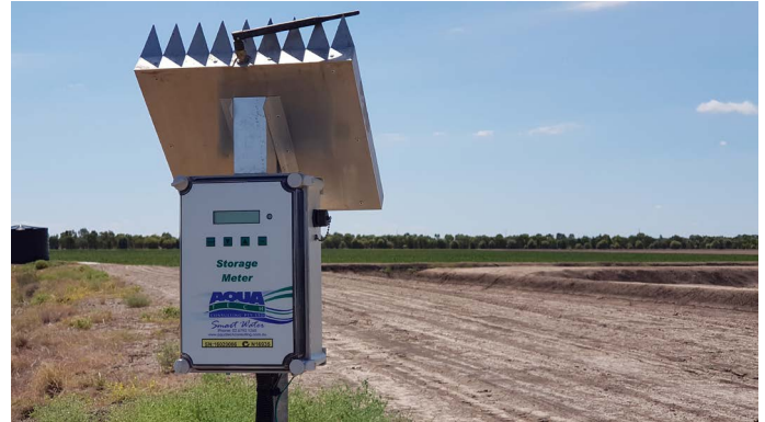
A storage meter can accurately analyse seepage and evaporation (Image: P. Verwey)
