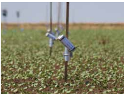
Canopy temperature sensors monitor the crop 24/7
