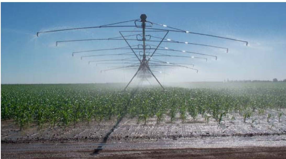
Spreader bars on a lateral move system irrigating corn to better match the application rate to the soil infiltration rate.
